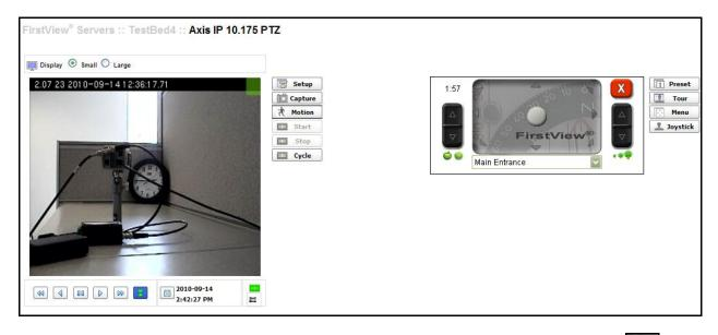
In addition to sliding the puck to move the camera, users can also click any of the gray arrows in the touch pad to tilt and pan the camera.
